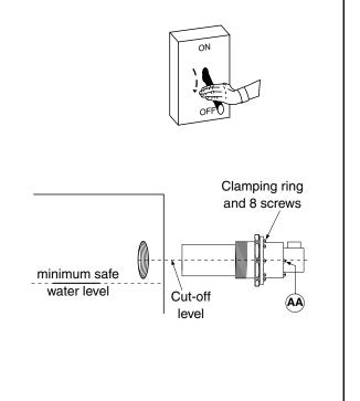
NOTE: To connect wires to the terminals on the water feeder, burner, or low water cut-off, place the bare end of the wire under the terminal screw and tighten the screw with a flathead screwdriver.
