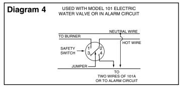
**IMPORTANT:** Low water cut-off circuit of the 69 series must be electrically wired in series with all other boiler limit operating controls.
