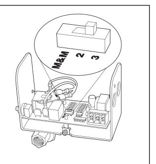
Connect a wire from the "Hot" side of the power supply to the water feeder terminal 3, and low water cut-off terminal 2. Connect a wire from the neutral side of the power supply to the water feeder terminal 2, and to the neutral side of the burner.
